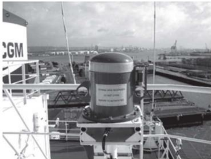
Figure 4: VDR on a ship in a protective capsule. ( http://www.marine-marchande.net , https://commons.wikimedia.org/w/index.php?curid=925946 .)
